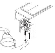
Figure O Sanitize Valve Body
